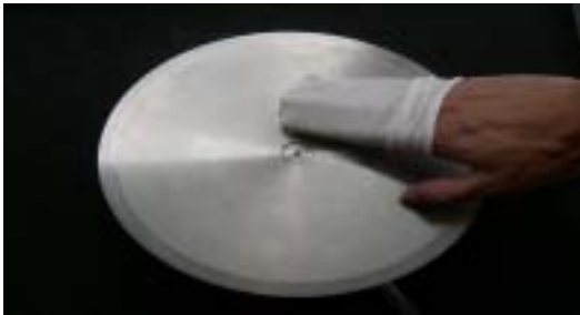
Figure 9: Clean the base plate with alcohol
