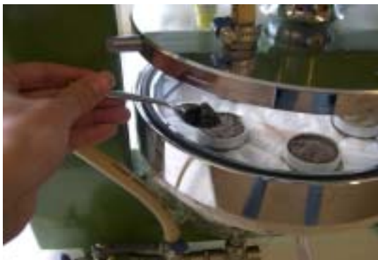
Figure 15: Use the spoon to fill the rings with soil
