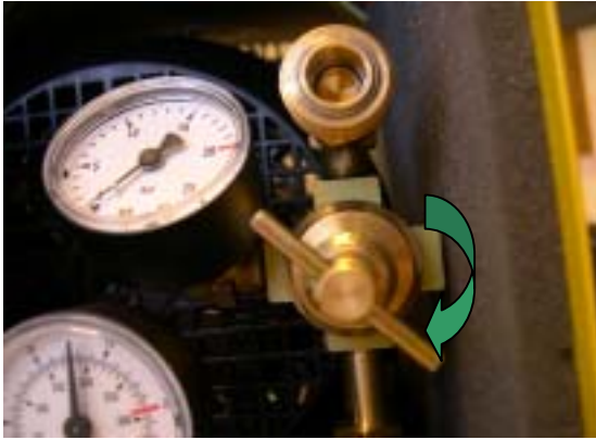
Figure18: Turn the control screw C
