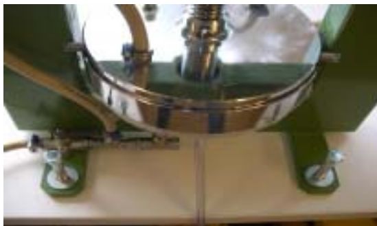
Figure 1: Secure to a table with bolts
