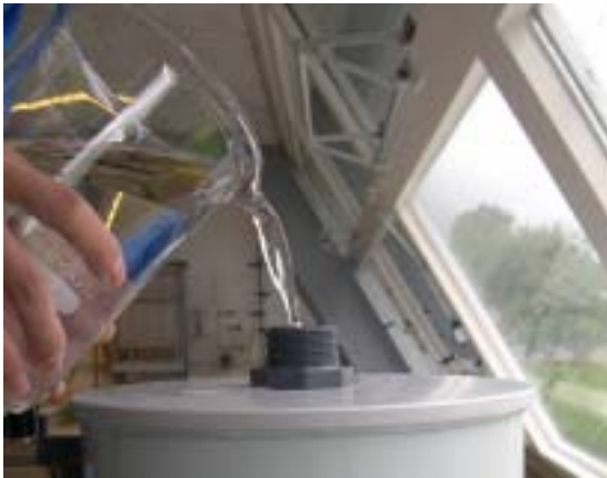
Figure 7 Fill the Vacuum Vessel with DM water
