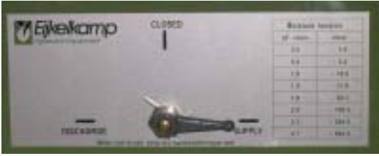
Figure 44: Tap A to supply
