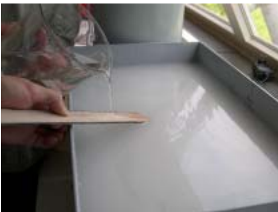
Figure 43: Gently add demineralised water
