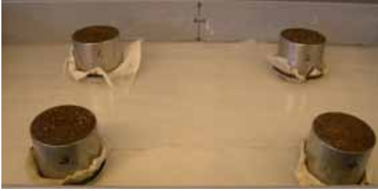
Figure 42: Wait for soil-water equilibrium
