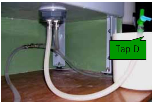
Figure 13: Air-bubbles released through Tap D
