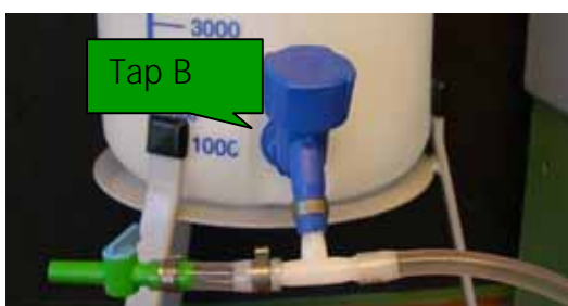
Figure 11: Turn Tap B 'On'.
