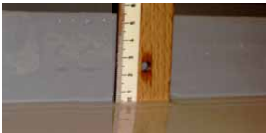
Figure 31: Retain 0.5cm water above sand
