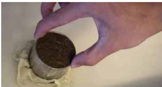
Figure 36: Press to ensure soil-sand contact
