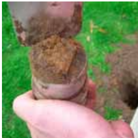
Figure 29: Chip off excess soil – don't smear!
