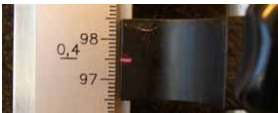
Figure 37: Pressure of -2.5 cm head (pF 0,4)
