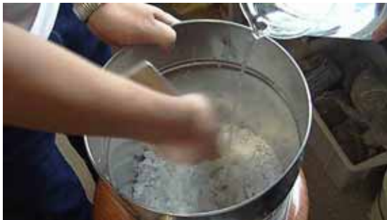
Figure 17: Saturate sand with water
