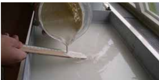
Figure 19: Adding water-saturated sand
