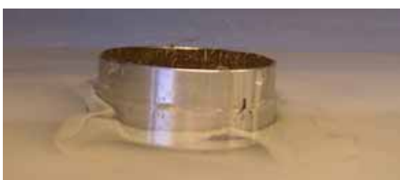
Figure 33: Saturate Sample (Water 1cm below top)
